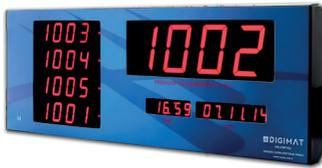
The Nurse Call Panel is an intelligent unit with a microcontroller RTC and E<sup>2</sup>. It can operate by itself or with a connection to a PC. Mode settings are available. It displays up to 5 calls at and displays the time, and date. The system communicates via RS485 modules. Other adjustments can be performed manually through a PC connection.
